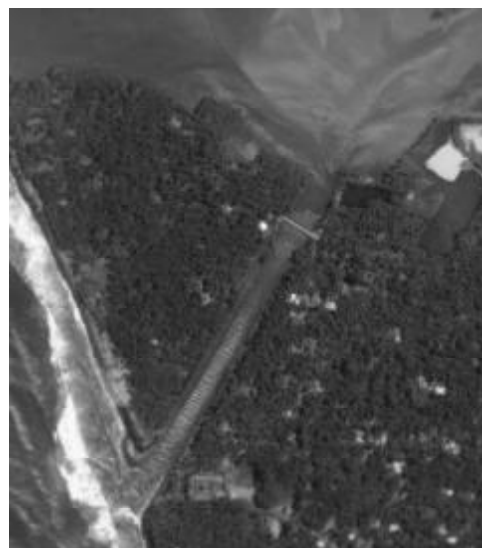
Fig. 1b: Digital globe satellite imagery from Google Earth clearly shows the buildup of sediment shoals in the Paravaur estuary close to the tidal regulator at Pozhikkara in Kerala, India
