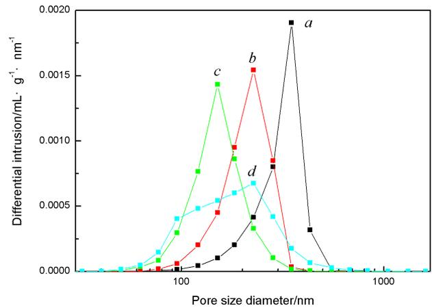
Fig. 2: Pore size distribution of DPC at different tourmaline content. a) 0%; b) 8%; c) 12%; d) 16%.
