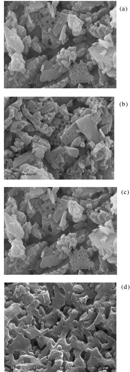
Fig. 1: SEM photograph of DPC in different tourmaline contents. a) 0%; b) 8%; c) 12%; d) 16%
