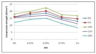
Fig. 2: Compressive strength of different mixes at 7 days.
