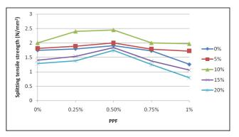
Fig. 5: Splitting tensile strength of different mixes at 7 days.
