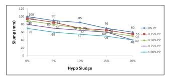
Fig. 1: Degree of workability of various mixes using slump test.
