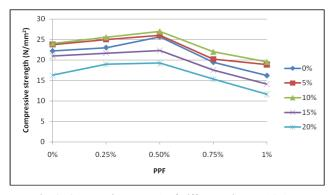
Fig. 3: Compressive strength of different mixes at 14 days.
