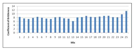
Fig. 8: Variation of coefficient of brittleness for different mixes at 28 days of curing.
