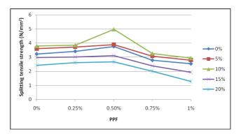
Fig. 7: Splitting tensile strength of different mixes at 28 days.
