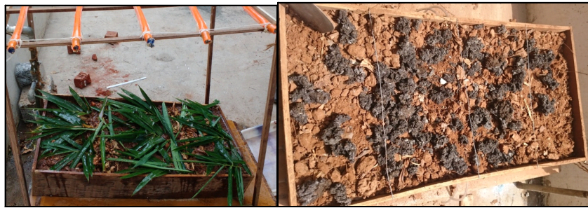
Fig. 2: Simulation of mulching and dewatered sludge covering for erosion control.
