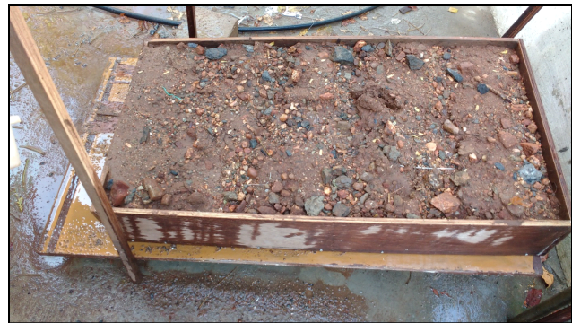
Fig. 3: Simulated soil erosion without any control measures.
