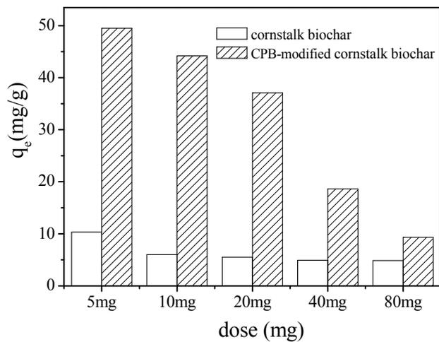
Fig. 2: Effect of the dose of the raw cornstalk biochar and CPB-modified cornstalk biochar on the uptake of ORII.
