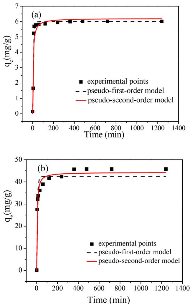
Fig. 4: Non-linear adsorption kinetic simulation for (a) pseudo-first-order and (b) pseudo-second-order models.
