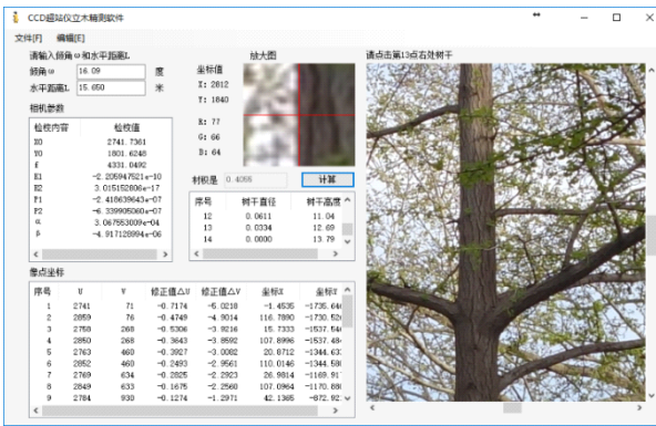
Fig. 3: CCD main interface of precise measurement software of standing tree based on CCD SmartStation.
