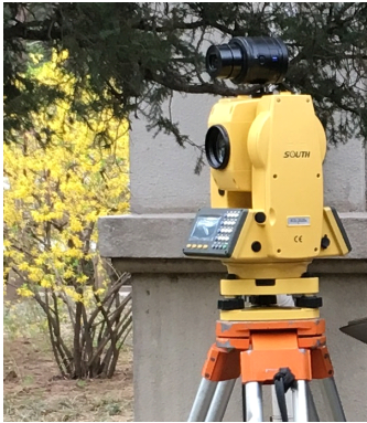
Fig. 2: Real product photo of CCD SmartStation.
