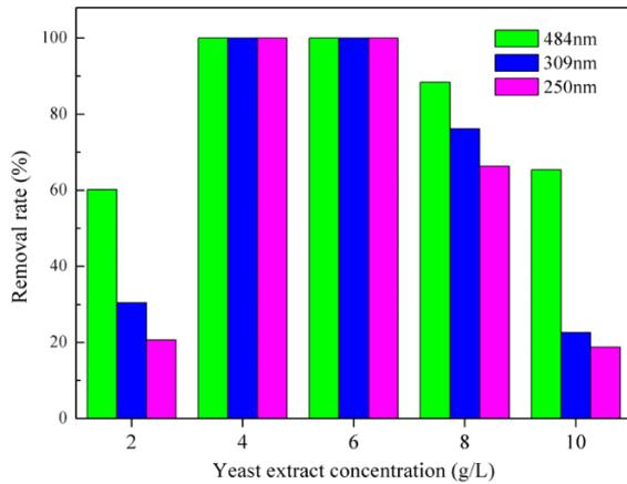
Fig. 4: Effect of yeast extract concentration on AO7 (20 mg/L) degradation.
