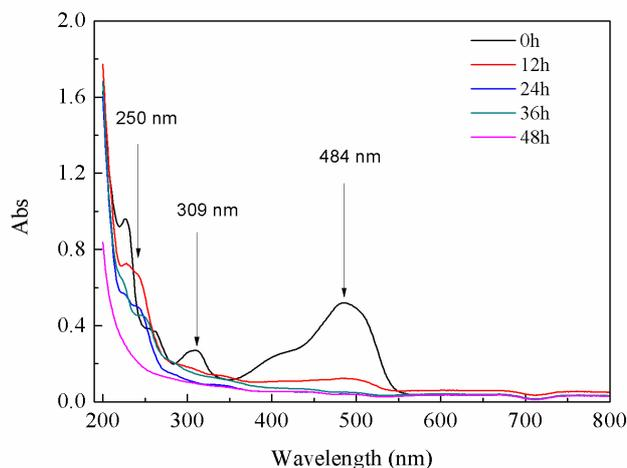
Fig. 1: UV-Vis spectra of AO7 and degraded products at varied time intervals under static and shaking condition at 30°C by mixed cultures.
