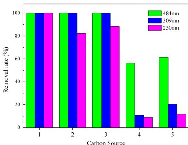
Fig. 2: Effect of various carbon sources on degradation of AO7 (20 mg/L) along with 5 g/L yeast extract. 1: no carbon source; 2: glucose; 3: sodium acetate; 4: sucrose; 5: starch
